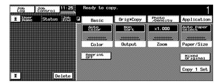
The Basic screen uses graphics and messages to show the currently selected settings, the modes and functions that can be selected, and the status of the machine.
